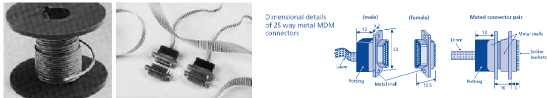
Figure 31: Oxford Instruments: a) stainless steel coaxial cable; b) ribbon cable; c) MDM metal connectors
