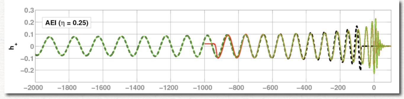
Red line is the numrel waveform Black dashed line is the 3.5PN waveform Green line is the hybrid waveform
