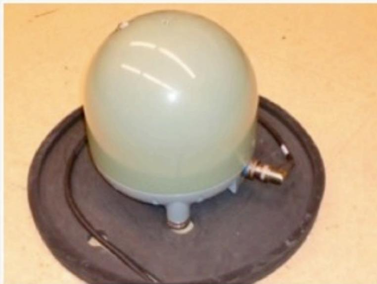
The seismometers are usually mounted on a hardrock tile (attached to the ground with concrete) and covered by an acoustic insulating cover. A thermal insulating box filled with insulation foam is then placed on top of the instrument to further isolate the instrument from external influences.
