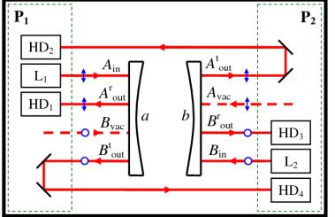
Double-pumped FP cavity is an example of partial DFI with the GW response  $\left(L/\lambda_{\rm GW}\right)^0 h$  (no resonant gain). Displacement noise of the cavity mirrors is canceled. Sensitivity is limited by laser noise and residual displacement noise of the optical benches.
