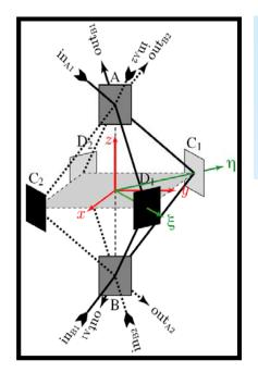
Linear combination of 4 responses is completely DNF and GW response is  $\propto \left(L/\lambda_{\rm GW}\right)^2 h$
