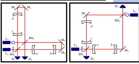
Double-pumped resonant speed meter is an example of partial DFI with the GW response  $\left(L/\lambda_{\rm GW}\right)^{\!\! 1}h$  with the resonant gain. It has laser noise suppressed (balanced scheme) but sensitivity is limited by displacement noise of auxiliary mirrors.
