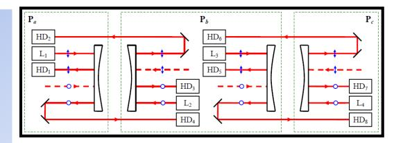
Two symmetrically positioned Michelson/FP interferometers is a balanced modification (laser noise free) of the two-cavities scheme. GW response is  $\left(L/\lambda_{\rm GW}\right)^2 h \approx 10^{-5} \times h$  for
