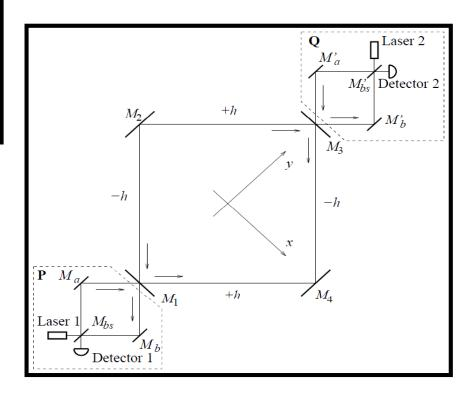
Two symmetrically positioned double-pumped FP cavities. Allow complete displacement noise cancelation with the resonantly amplified  $\left(L/\lambda_{\rm GW}\right)^2 h$  response.
