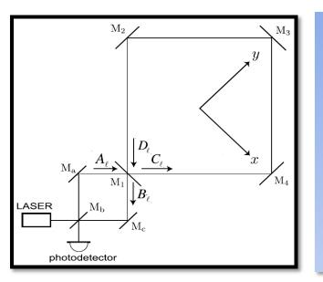
Sagnac-type interferometer is not sensitive to the motions of the input and "end" mirrors at all frequencies, because clockwise and counterclockwise optical waves encounter them simultaneously.
