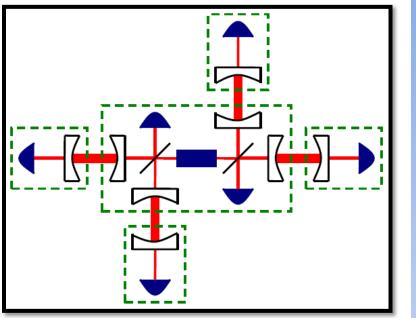
To cancel the noise of the central platform the second interferometer is positioned symmetrically.
