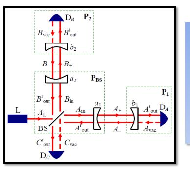
A single Michelson/FP interferometer with partially transmittable end-mirrors. Both reflected and transmitted waves are monitored. Transmitted waves are registered with the homodyne detectors.
