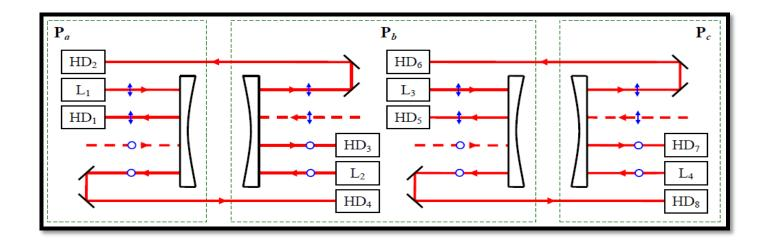
Three platforms with *rigidly mounted* lasers, photodetectors and cavities mirrors. Both cavities are pumped from both sides. An experimentalist monitors either reflected signals or transmitted ones.
