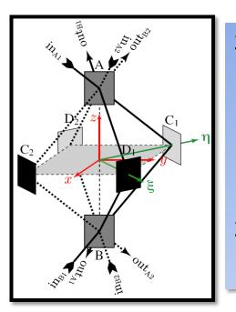
3D DFI (Octahedron) is composed of 4 Mach-Zehnder interferometers. The proper linear combination of their responses cancels displacement noises of all mirrors and beamsplitters. The GW response has the order of  $h(L/\lambda_{GW})^2=10^{-5}h$  for L=10 km and  $f_{GW}=100$  Hz.
