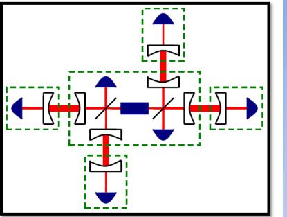
To cancel the noise of the central platform the second interferometer is positioned symmetrically.
