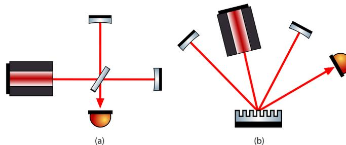
Figure 1: Michelson and reflection grating beam-splitter options. (a) Traditional Michelson interferometer design with 4 port beam-splitter and (b) 4 port, all-reflective beam-splitter configuration.
