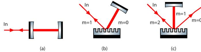
Figure 2: Traditional cavity and reflection grating cavity configuration comparison. (a) Traditional Fabry Perot cavity design with 2 port mirror coupler, (b) 2 port, 1st order Littrow mount cavity input coupler and (c) 3 port, 2nd order Littrow mount cavity coupler.
