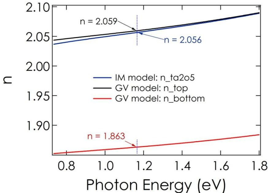
The value of  $n$  seems to be substantially model-independent: its value is determined with an uncertainty of a few parts per mil and it is in excellent agreement with the value  $n_{\text{LMA}} \approx 2.06$ , obtained by LMA.
